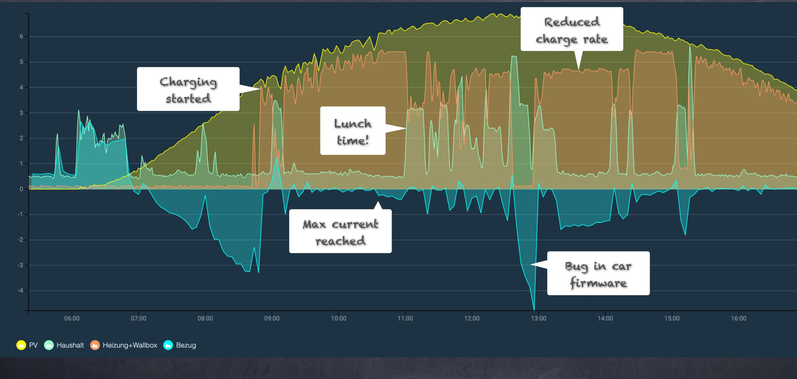
25 kWh from grid, 5 kWh to grid, 25 kWh to car (2150 km)
